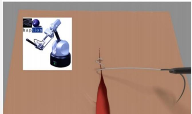
Virtual suturing task; the needle holder is controlled via Virtuouse 6D Desktop
