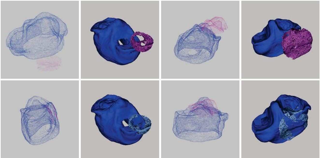
Fig. 6: Examples of erroneous registration results. The initial positions of the template with respect to the target are shown on the top row. The corresponding unsuccessful registration results with convergence  $score > 2mm$  are shown on the bottom row (from left to right: ICP, optimal step non-rigid ICP, CPD, diffeomorphic non-rigid).
