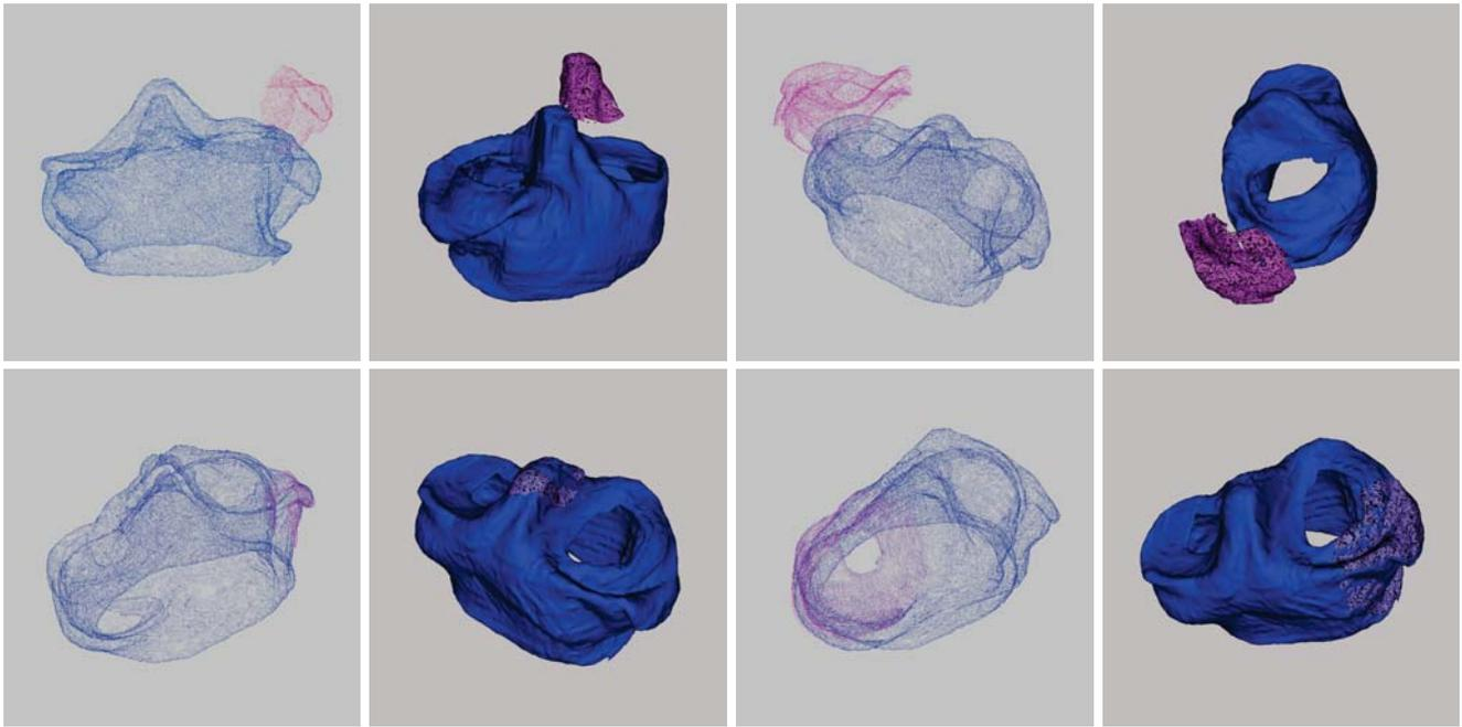
Fig. 5: Examples of good registration results. The initial positions of the template with respect to the target are shown on the top row. The corresponding successful registration results with  $RMSError < 10^{-3}mm$  are shown on the bottom row (from left to right: ICP, optimal step non-rigid ICP, CPD, diffeomorphic non-rigid).
